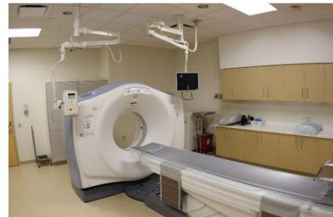
Figure 19 - A CT scanner ( source ).
